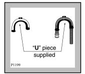
Place the drain hose into your standpipe, which should have an internal diameter of approximately 38mm thus ensuring there is an air break between the drain hose and standpipe.
